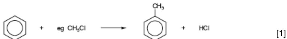
accept C<sub>6</sub>H<sub>5</sub> in place of the ring accept equations that show the catalyst
